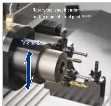
**Opposite tool post equipped with a Y2 axis**
